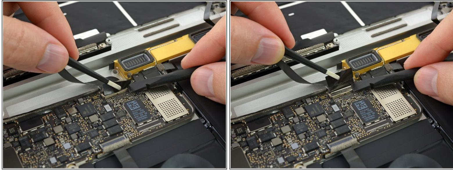
*(i)* It's possible the metal retaining flap on the display cable connector may flip open, remaining stuck to the tape.
